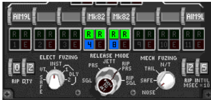
4 and 8 selected, rippling pairs all the R lights are on, a pair will drop, then another
