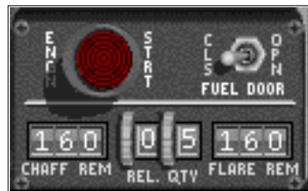
Chaff and flare controls
